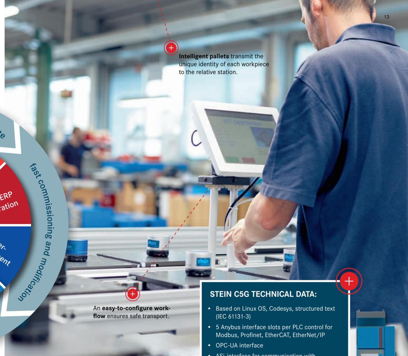
**+** **Intelligent pallets** transmit the unique identity of each workpiece to the relative station.
