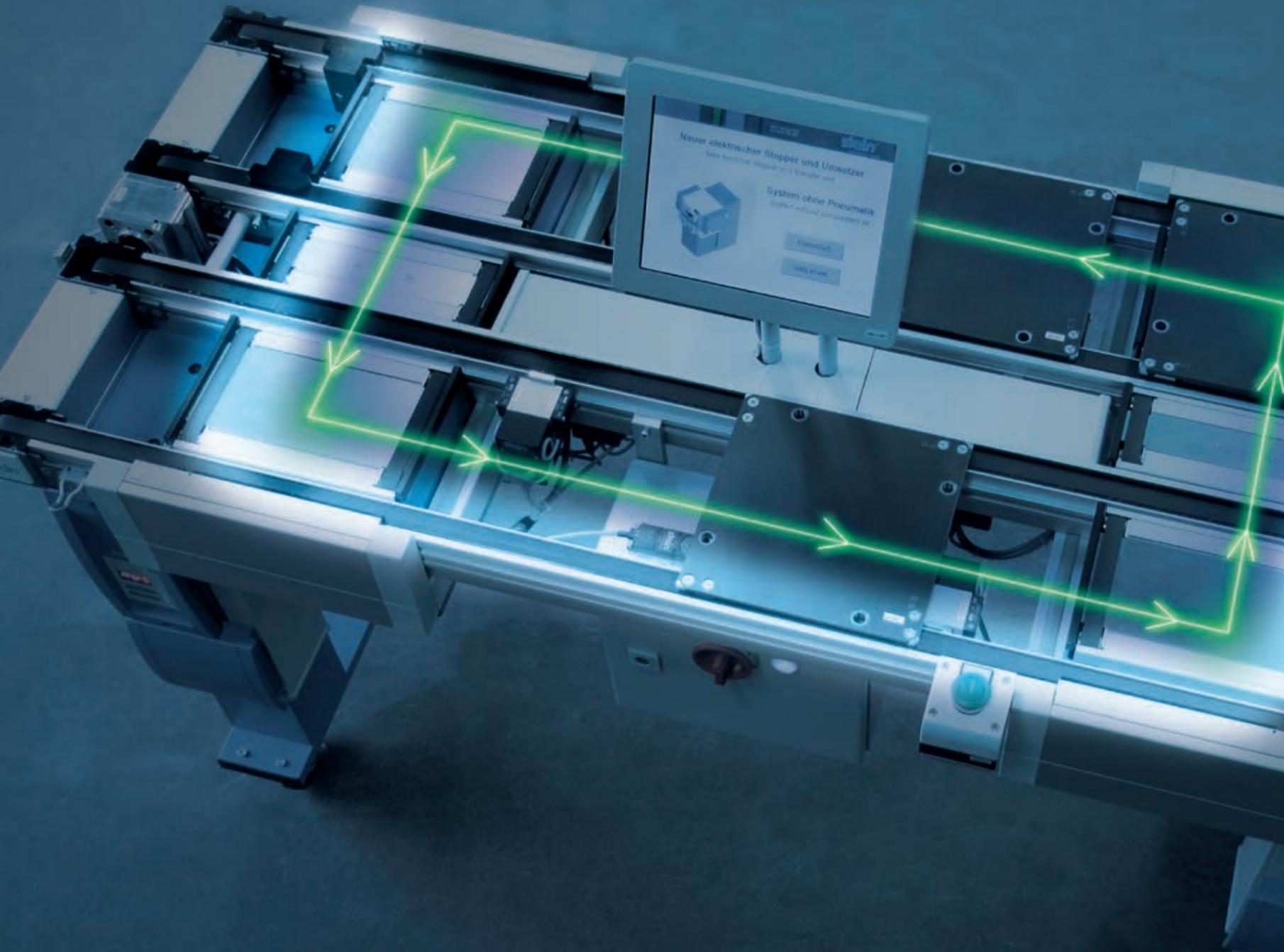
STEIN supports the trend towards electrification with the purely electric version of the 300 system - STEIN 300e. Instead of pneumatics, the stoppers, transfer units or centering devices are controlled via electric drives. This is particularly a big advantage for cleanroom applications. As a side benefit, STEIN 300e is even more energy-efficient than STEIN 300 already is.
